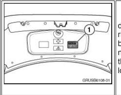
d. Install a warning label (PN 71 24 6 777 721) on the right side of the tool kit cover (1). The customer should be notified of the label and the fact that liquids should not be present on or under the trunk insulation, due to the sensitive nature of the electronic control units located in the spare tire well.
